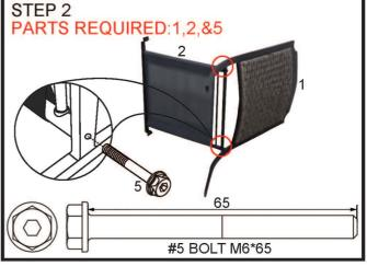
Use the correct bolts as indicated. Do not tighten any of the bolts until the chair is completely assembled.
