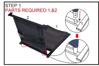
Use the correct bolts as indicated. Do not tighten any of the bolts until the chair is completely assembled.
