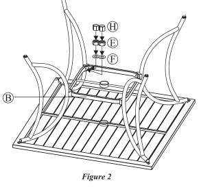
Step 4: After making any necessary adjustments to the alignment of the table base and table top, use the hex bolt driver and hex wrench to tighten all bolts and nuts.
