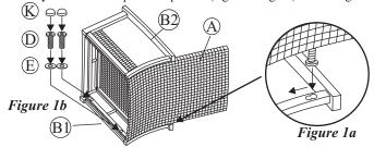
**Step 3:** Place the swivel base (with rocker assembly) on a flat, solid surface. Make sure the rocker assembly is positioned all the way into the base. It may have shifted or vibrated out during shipment.
