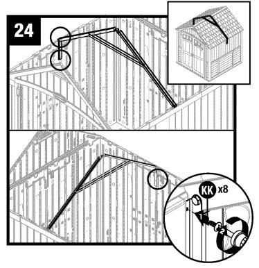
Secure with four screws (KK) in each side adaptor bracket
