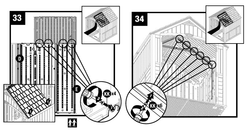
Pull down each lower corner of roof from outside. From inside shed, attach tabs on side panel (D) and right front (E) corner to roof panel with four screws (KK).
