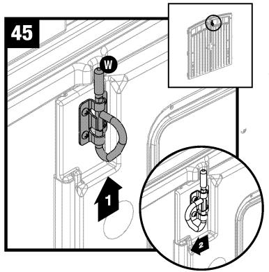
Push D-ring (W) up to engage with slot in header. Turn D-ring to left for locked position. Repeat with lower D-ring.
