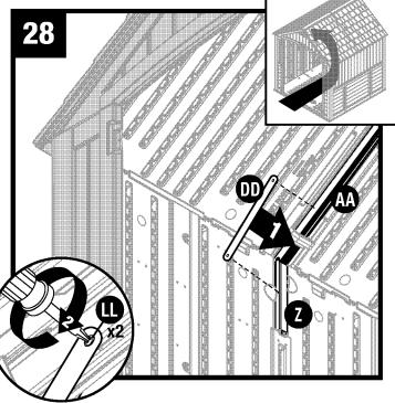
Attach truss strap (DD) to left truss tie down (Z) and truss leg (AA). Secure with two screws (LL).
