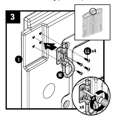
At top interior side of left door (I), attach D-ring slide bolt (W) with four screws (LL) through provided holes.
