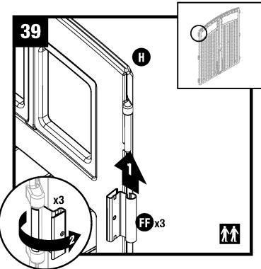
Stand right door (H) upright with three hinge mounts facing right. Slide one metal hinge plate (FF) up onto each hinge mount. Rotate hinge plates to outside of door. Snap metal hinge plate into place by pushing towards door.
