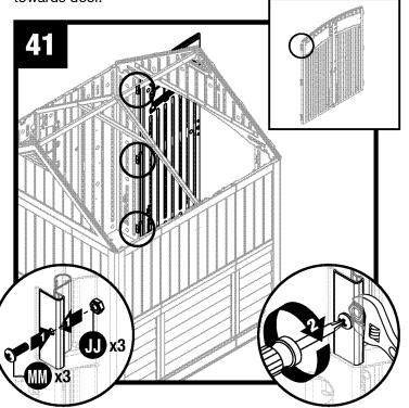
Secure each metal hinge plate with one screw (MM) and one nut (JJ).
