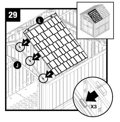
Lay right roof (L) directly over three tabs on right side of front header (J). With right roof channel seated over/on header tabs, check alignment in all three spots.
