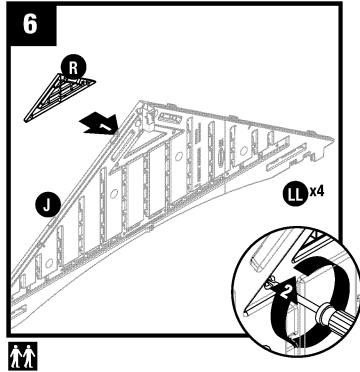
Place header vent (R) into front opening in front header (J). Secure through back of header with four screws (LL). **DO NOT** over tighten screws.
