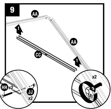
Attach truss cross beam (CC) to two truss legs (AA) using two hex head cap screws (HH) and two nuts (JJ). Stand truss and check cross beam is level.
