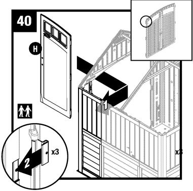
With door hinge in open position, slide one door hinge over each hinge receptacle on inside of right front corner.
