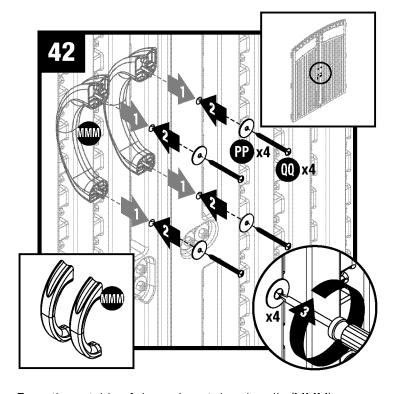
From the outside of doors, insert door handle (MMM) stems into holes of left and right doors. On inside of doors, place washers (PP) on each door handle stem, and secure each with one screw (QQ).
