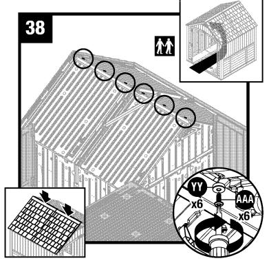
Push down the roof from outside. From inside shed, secure roof panels together along ridge of roof using six rubber washers (YY) and six sealing screws (AAA).
