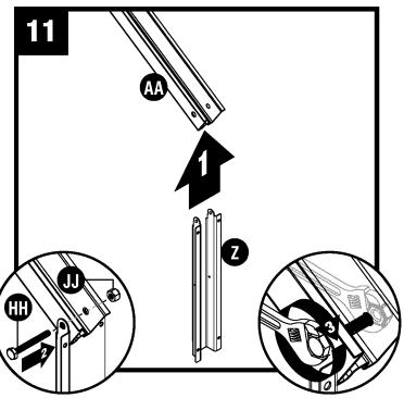
Place side adaptor bracket (Z) at end of right truss leg (AA). Secure adaptor bracket with one 2" hex head cap screw (HH) and one nut (JJ).
