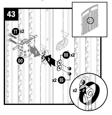
Insert two screws (TT) into door latch assembly (OO) and through right door. While holding plate in place on exterior of door, secure each screw with two washers (RR) and two locking nuts (SS).
