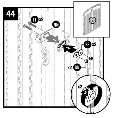
Insert screws (TT) into left latch plate (NN) and through left door. While holding plate in place on exterior of door, secure each screw with two washers (RR) and two locking nuts (SS).
