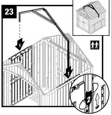
Slide truss assembly into place.
