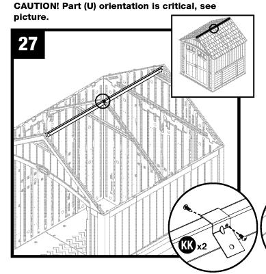
Attach the roof truss assembly to the ridge beam with two screws (KK).
