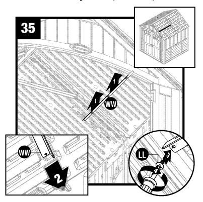
Raise roof support (WW) into position against roof. Slide roof support (WW) into front header. Secure roof support (WW) to underside of truss leg with one screw (LL).
