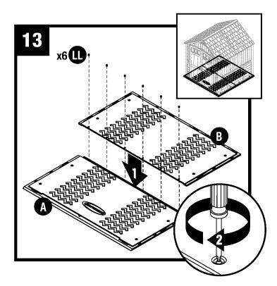
Push front floor (A) and rear floor (B) panels together and secure with six screws (LL).
