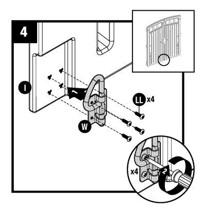
At bottom interior side of left door (I), attach D-ring slide bolt (W) with four screws (LL) through provided holes.
