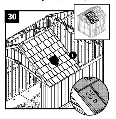
Slide right roof (L) down towards the outside of shed. You will hear a "snap" when engaged.
