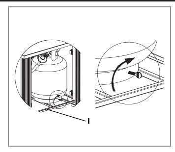
8. Turn the cylinder valve on the tank clockwise to close the propane tank. Attach the preassembled regulator from the table top (B) to the cylinder valve by turning the regulator coupling nut clockwise. Make sure it is fastened securely and tighten connections by hand only.
