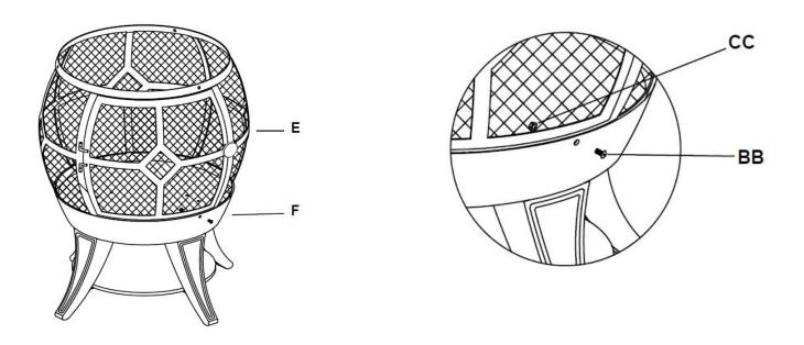
**Step 5:** Attach the chimney top (D) to the mesh screen (E) using  $M6 \times 25$ mm bolts (BB) and M6 nuts (CC). Securely tighten each bolt (BB) and nut (CC) with an M6 wrench and Philips screwdriver (not included).
