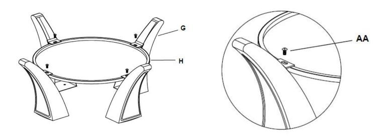
**Step 3:** Attach the chimney bottom (F) to the stand (G) using  $M6 \times 12$ mm bolts (AA). Securely tighten each bolt (AA) with a Philips screwdriver (not included).
