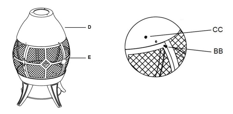
**Step 6:** Attach the chimney flue (C) to chimney top (D) using  $M6 \times 25$ mm bolts (BB) and M6 nuts (CC). Securely tighten each bolt (BB) and nut (CC) with an M6 wrench and Philips screwdriver (not included).
